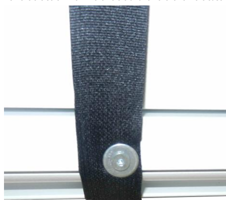
Remove the screw which fix the Velcro and remove it from the case:
