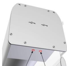
HOLES FOR END STOP LIMIT
